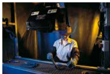
Magnaflux Crack Detection
