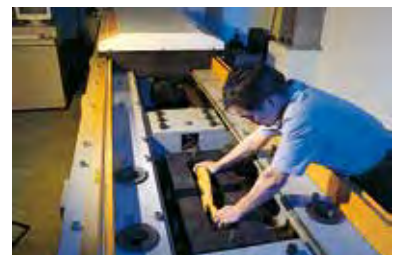
Tensile Test, Capacity 300 tonnes
